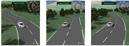
Figure 13: CarMaker simulation for lane keeping experiment
